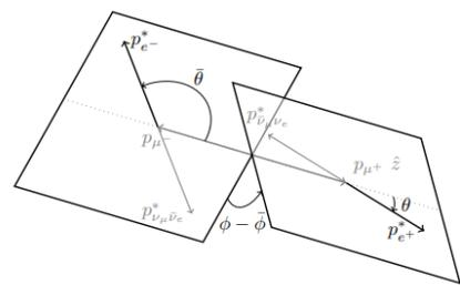
FIG. 11. Kinematics of the process. The decaying muons' momenta in the  $\eta$  rest frame are noted as  $p_{\mu^\pm}$ , while the  $e^\pm$  momenta,  $p_{e^\pm}^*$ , is shown in the corresponding  $\mu^\pm$  reference frame along with the momenta of the  $\nu\bar{\nu}$  system. The  $\hat{z}$  axis is chosen along  $p_{\mu^+}$ .
