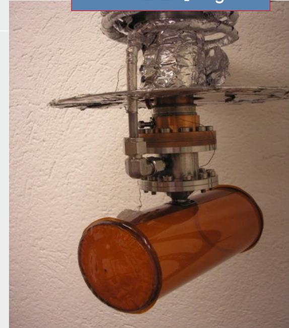
*Target for  $p$  and  $\pi^+$  beams: 10x 0.78 mm Li or Be foil*
