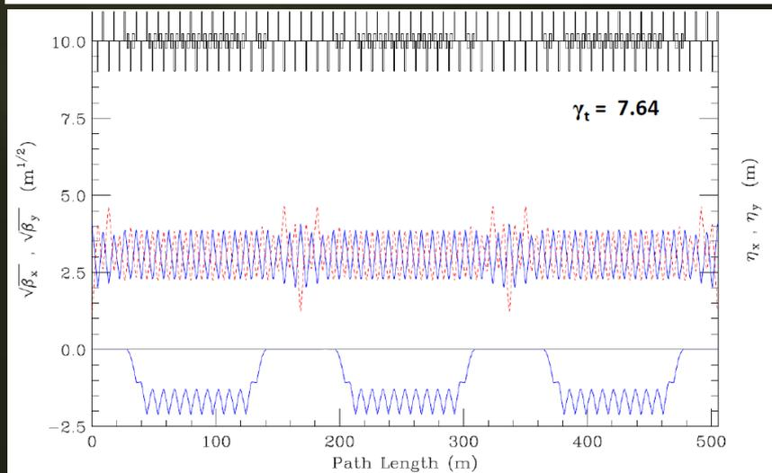
8 GeV injection energy (top) and <5.8 GeV (bottom)
